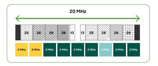
Uplink and downlink orthogonal frequency-division multiple access (OFDMA) increases network efficiency and lowers latency for high-demand environments.
